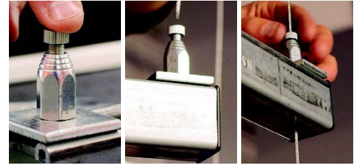
depress plunger insert wire rope tighten collar to lock
