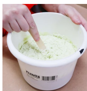
Mix the solution slowly and take care to avoid creating air bubbles
