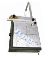
Proxxon Thermocut Bench Cutter Ideal for architectural and theatre modelmakers. The 390 x 280 mm working surface is of aluminium CoBond compound. This eases the pushing of work pieces. The table top has a printed grid and protractor. Supplied with a dual function fence with lockable feed bar. The throat depth is 350 mm and the machine will cut material up
